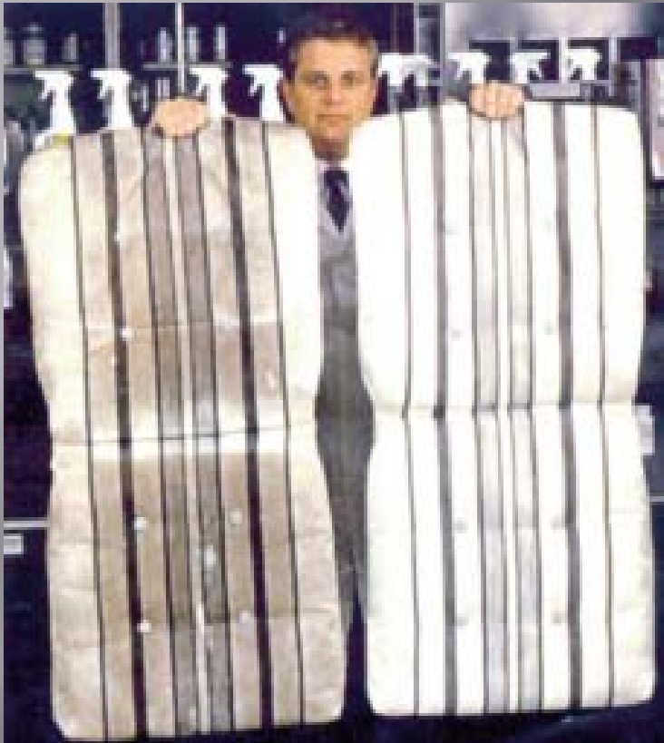
SurfaceGuard90 after 2 years of outside exposure
